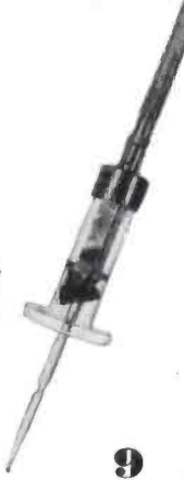
The finished filament-grid unit is ready to be assembled with the rebuilt anode and glass envelope.
