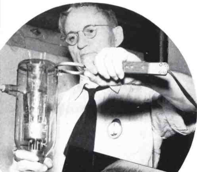
1 The glass envelope is carefully cut open by means of an electrically heated wire and application of a damp cloth.
