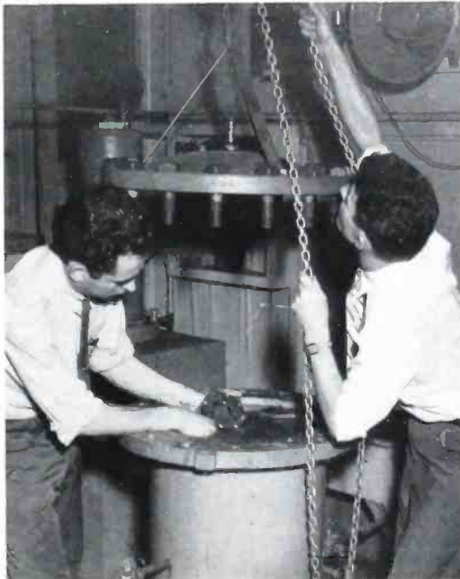
"20,000 LEAGUES UNDER THE SEA" is reproduced by this pressure tank developed to test RCA equipment destined for under-water duty. The equipment being tested is "submerged" in 600 feet of water for twelve hours and under pressure equivalent to 300 pounds per sq. in.
