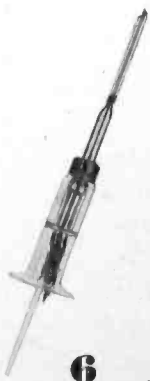
The completed rebuilt filament stem with new filament installed.
