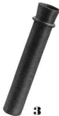
Rebuilt anode with new, thick copper cone ready for machining to obtain new feather-edge for glass-to-metal seal.
