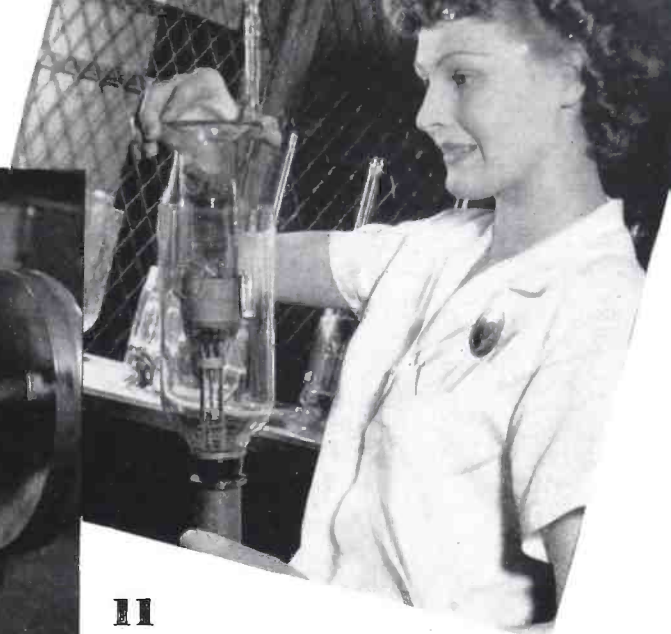
Checking the alignment of the filament-grid and anode-envelope assemblies before the glass filament stem is sealed to the glass envelope.
