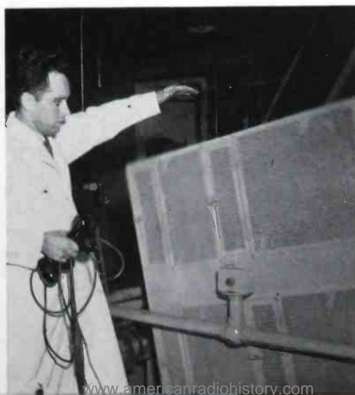
ACROBATIC GYRATIONS are provided by this device which is called the "tumbler" test. In rotating the box the piece of equipment inside is dropped over 1,000 times. It is then checked to see that it still performs satisfactorily. Subsequent demands of battle conditions are adequately met by equipment which has passed this rigid test.
