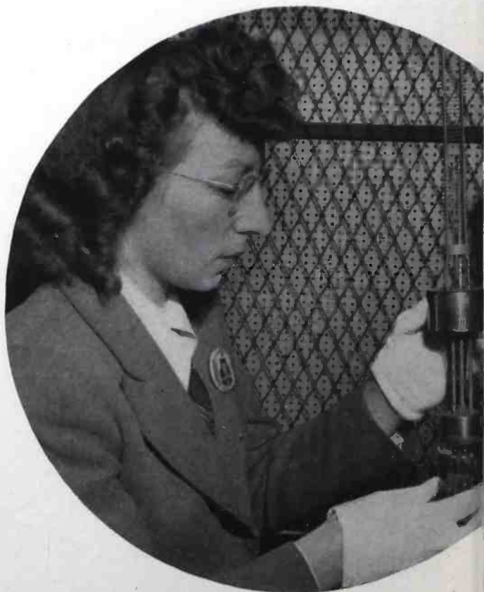
8 The grid structure is then mounted on the filament sub-assembly.
