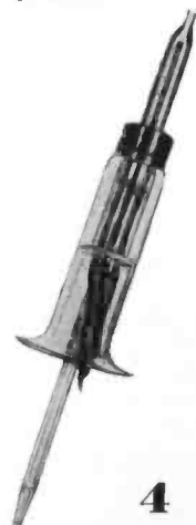
The old filament stem assembly is completely renovated. If the glass stem is cracked, the tungsten leads are salvaged and used to rebuild a new stem assembly.
