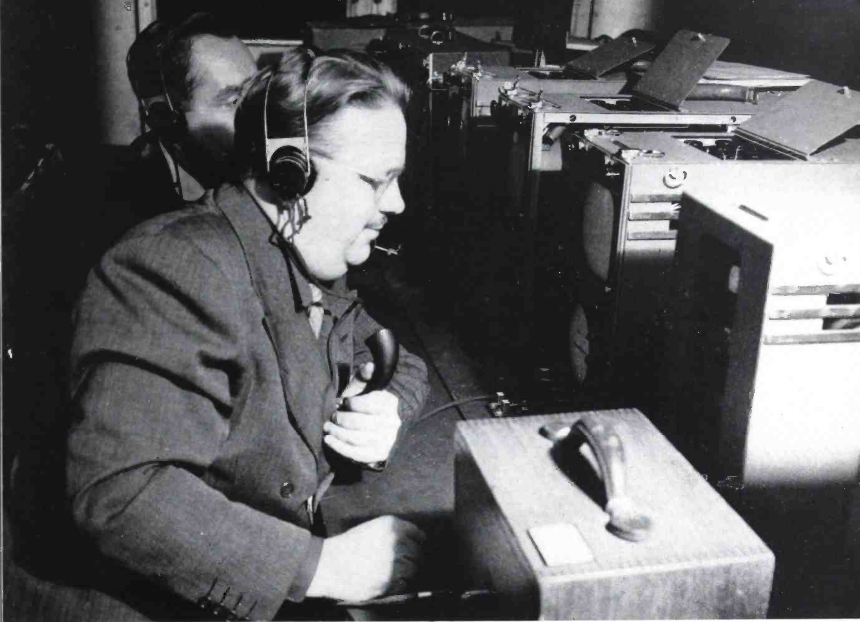
REMOTE TELEVISION PICKUP —Monitoring and switching equipment used by NBC in the rodeo broadcast and other remote pickups is shown mounted in the truck as actually used in this broadcast. With this equipment the cameras (as many as four) may be located up to 500 feet away. For further details see the article beginning on Page 20 of this issue.
