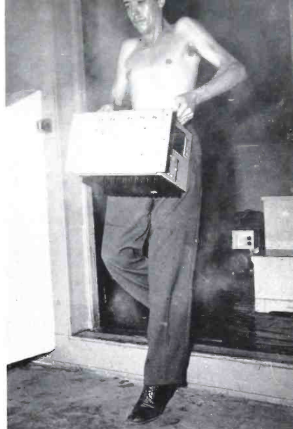
READY FOR THE "GREEN HELL" is the radio apparatus tested in the RCA laboratory "sweat-room" in which equipment is exposed to steam-saturated atmosphere at 60° C. (140° F.) and 95% humidity. Heat-laden moisture is a deadly enemy of electrical installations; yet the radio apparatus of America's fighting planes and bombers MUST function perfectly in landing fields and dispersal areas hacked from the "green hell" of Pacific jungles. Equipment tested in this manner is prepared for the ordeal of rain-drenched Guadalcanal or New Guinea.
